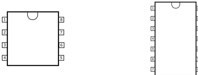
Figure 1.7: 8-pin and 14-pin IC chip outline.
